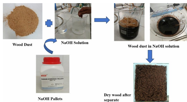
Fig. 1 : Wood Treatment Process.
